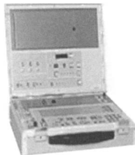
Figure 3.22 Torsional vibrometer (source: Ono Sokki, Japan Technical Report, website)
