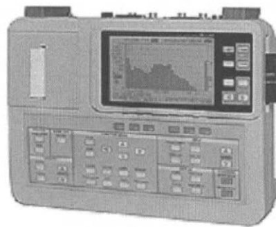
Figure 4.31 Real-time octave band analyzer (source: Ono Sokki, Japan website)
