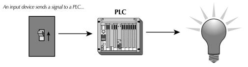
... An output device receives a signal from a PLC.
