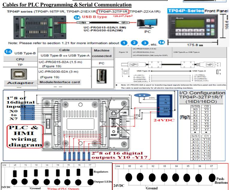
Delta PLC/HMI Cable Selection Guide
